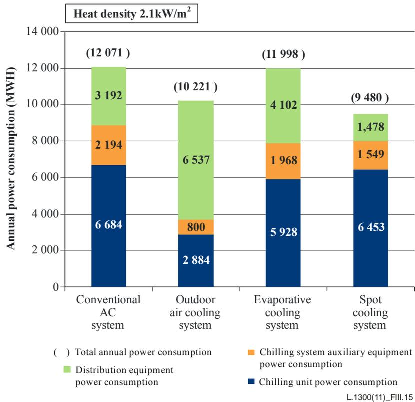
**Figure III.15 – Comparison of annual power consumption with air conditioning methods in Tokyo**
