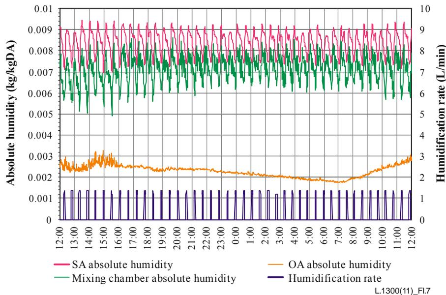
**Figure I.7 – Absolute humidity of air and the humidification rate**
