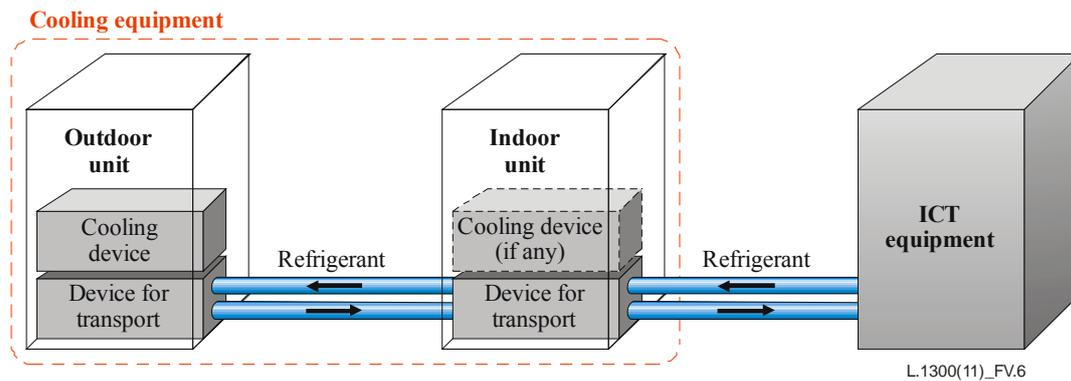
**Figure V.6 – General configuration of cooling equipment**
