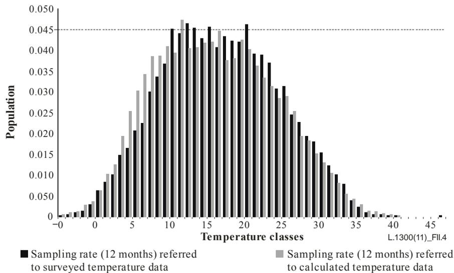
**Figure II.4 – Comparison between calculated and surveyed yearly temperature distributions**
