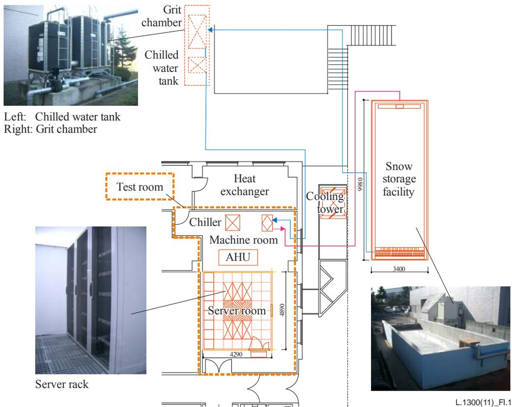
Figure I.1 – Layout of the test facility
