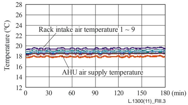
**Figure III.3 – Example of air conditioning in an outdoor air cooling system**
