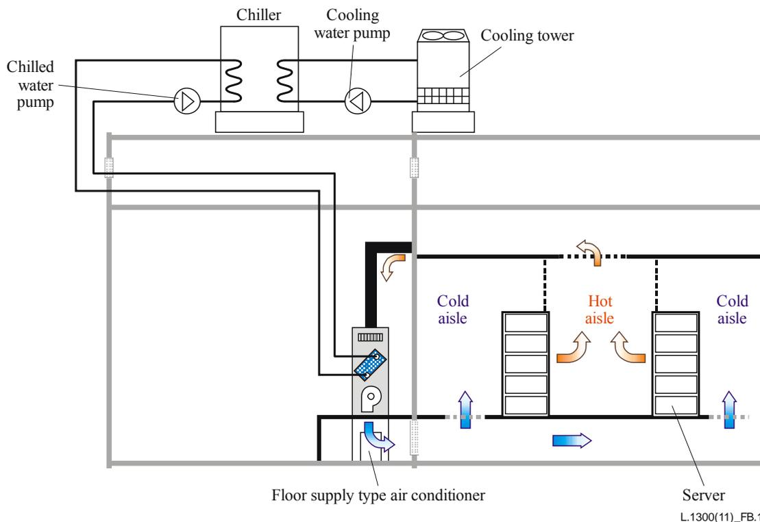
Figure B.1 – Conventional air conditioning system
