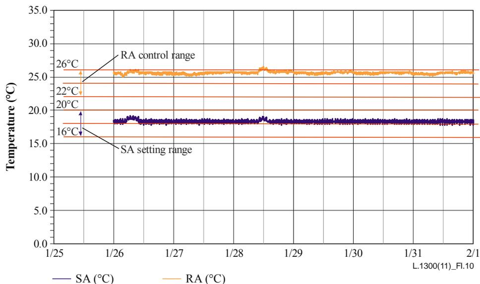
**Figure I.10 – Air temperature in snow and ice cooling**
