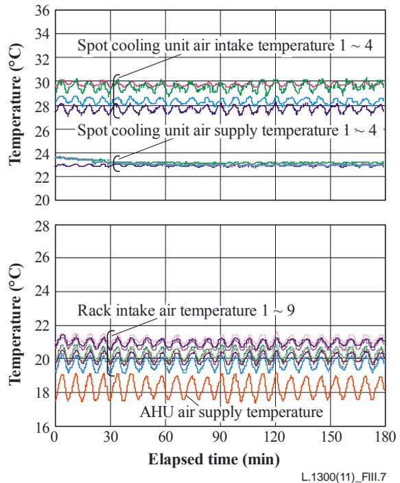
**Figure III.7 – Spot cooling method operational state (example)**
