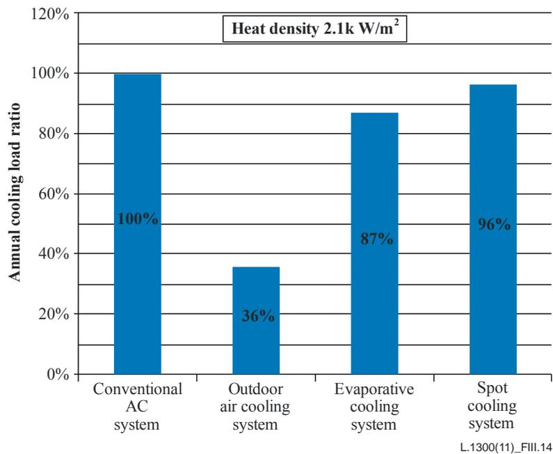
**Figure III.14 – Comparison of annual cooling load ratio with air conditioning methods in Tokyo**
