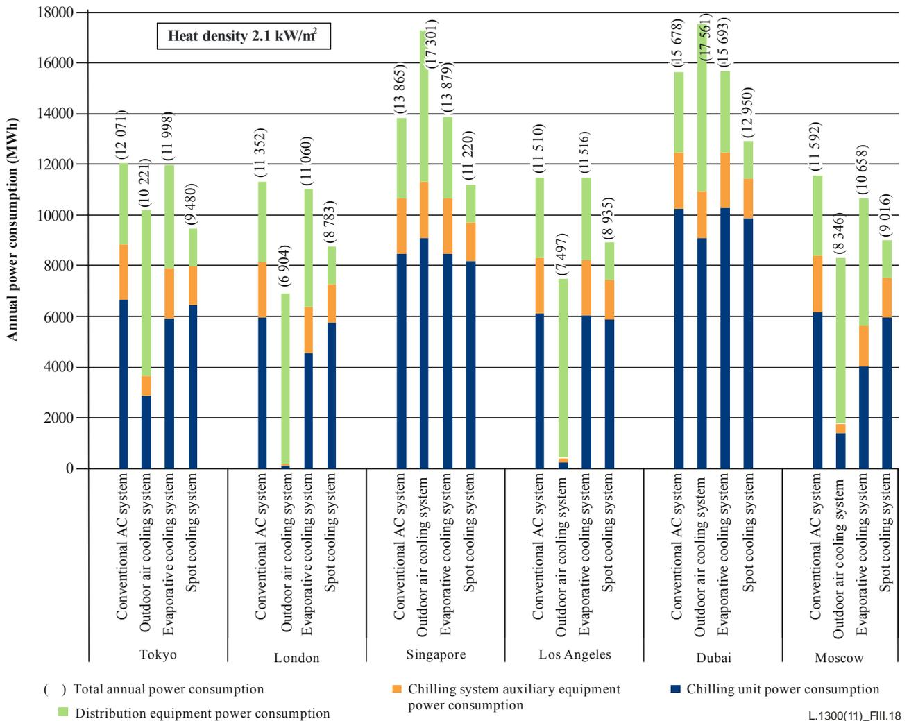
**Figure III.18 – Comparison of annual power consumption with air conditioning methods in six cities**
