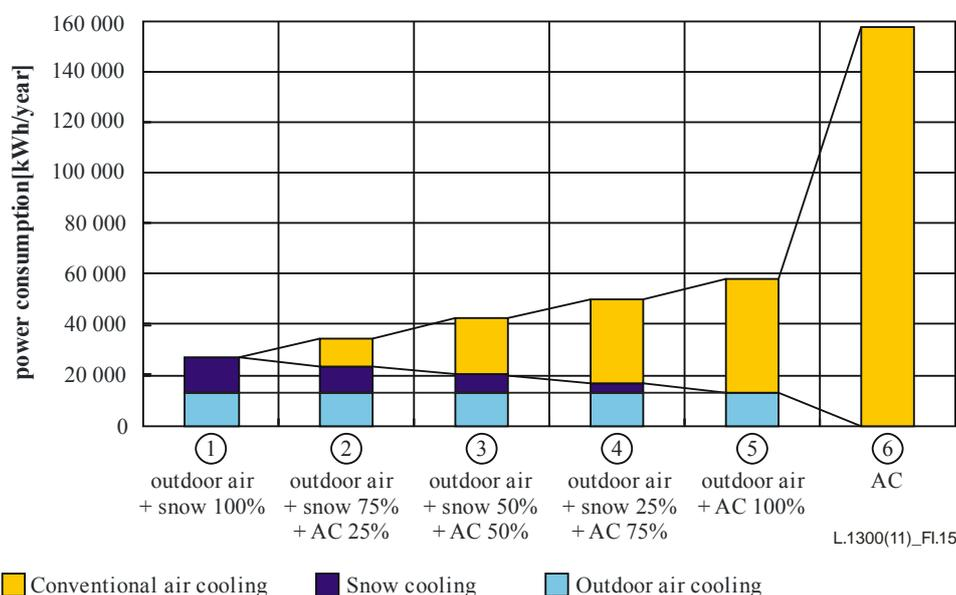
**Figure I.15 – Calculated annual power consumption of the test facility**
