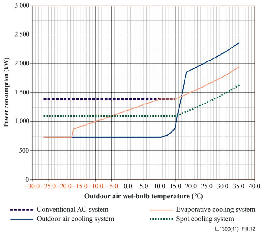
**Figure III.12 – Comparison of power consumption with outdoor air conditions (Heat density 2 kW/m<sup>2</sup>)**
