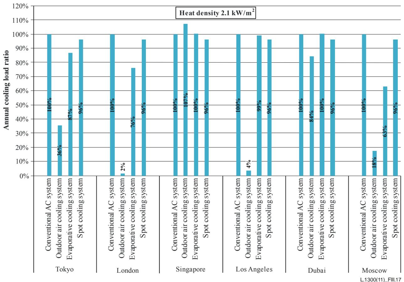
**Figure III.17 – Comparison of calculating results of annual cooling load ratio with air condition methods in six cities**
