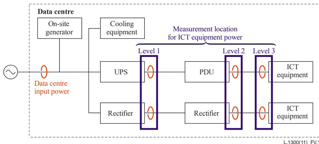
**Figure V.1 – Example of a power feeding system of a data centre**
