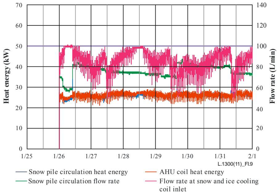
**Figure I.9 – Chilled water flow rate in snow and ice cooling**
