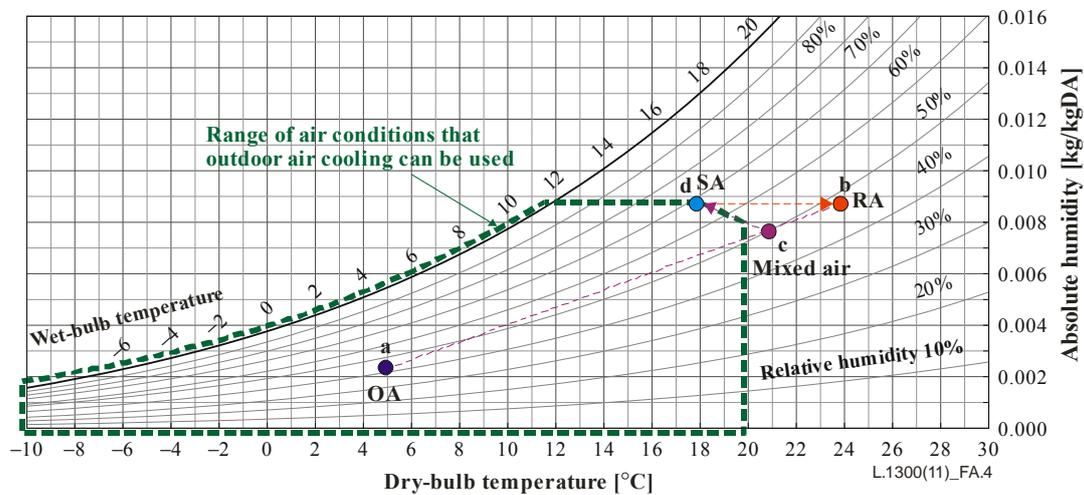
**Figure A.4 – Changes in air condition during outdoor air cooling**
