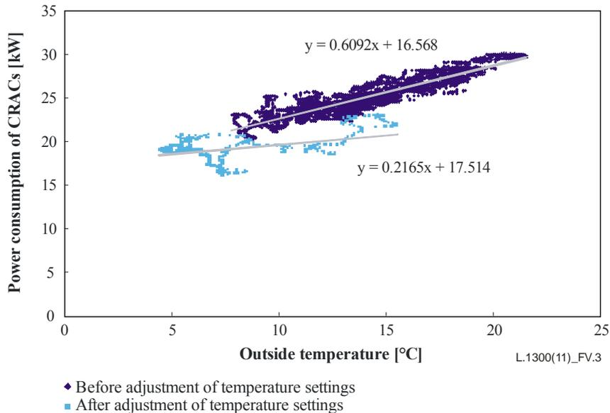
**Figure V.3 – Correlation of outside temperature and energy consumption of CRACs**
