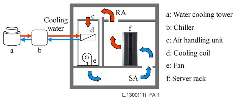
Figure A.1 – Air conditioning system components at a data centre
