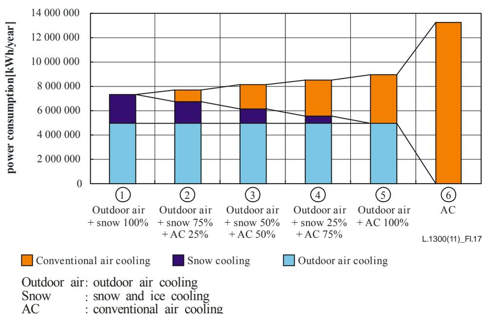
**Figure I.17 – Calculated annual power consumption of the 1000-rack model data centre**
