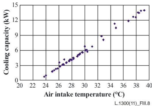
**Figure III.8 – Air intake temperature and cooling performance**
