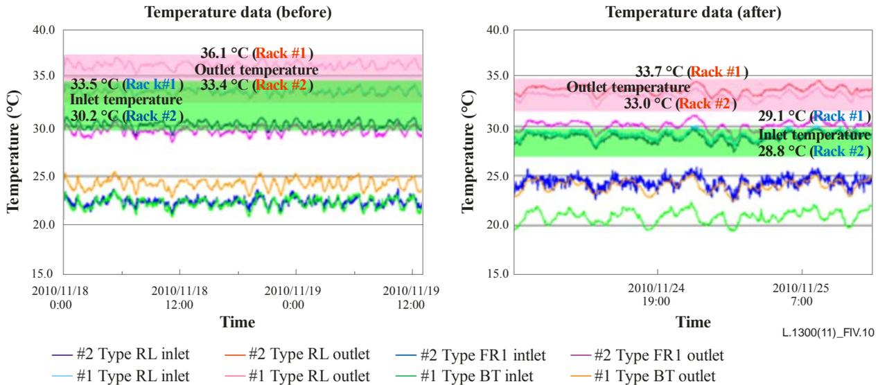
**Figure IV.10 – Results of Rack 1 after installing a plate at the outlet and at the inlet**
