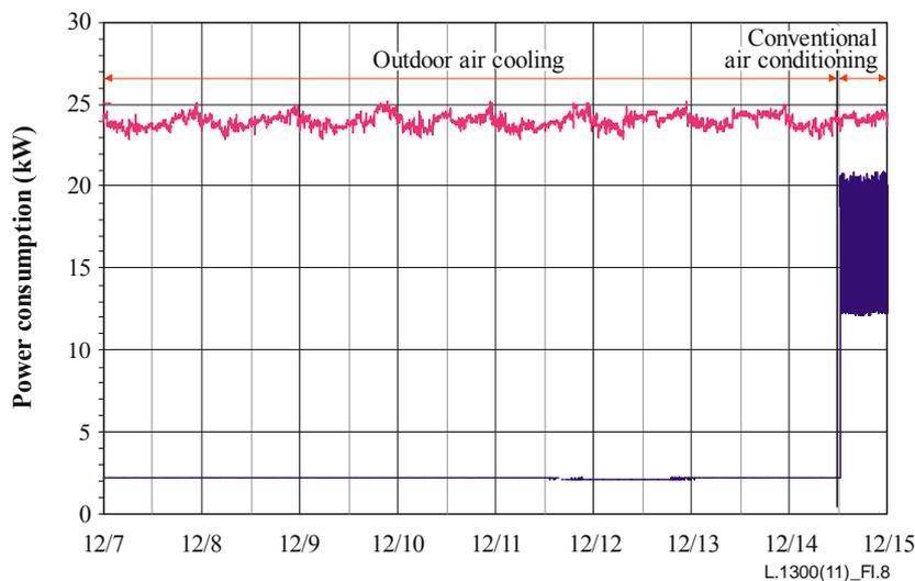
**Figure I.8 – Power consumption of servers and air conditioning equipment**
