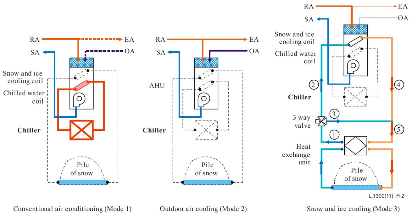
**Figure I.2 – Image of each cooling mode**
