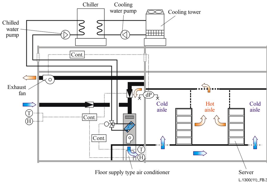
**Figure B.3 – Outline of an outdoor air cooling system**
