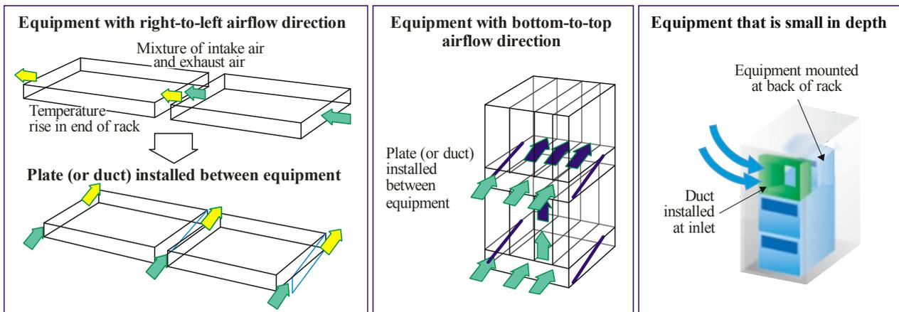
Figure IV.1 – Examples of types of rack mount equipment in which airflow correction is necessary
