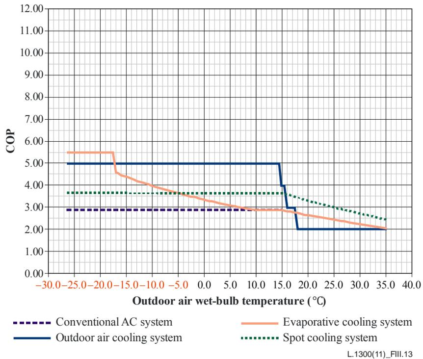
**Figure III.13 – Comparison of COP with outdoor air conditions (Heat density 2 kW/m<sup>2</sup>)**
