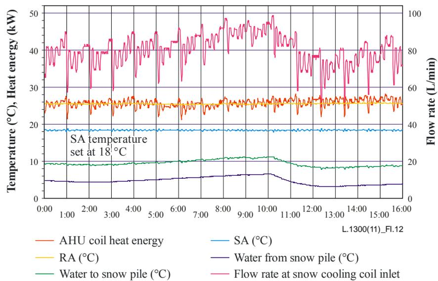
**Figure I.12 – Air temperature in snow and ice cooling**
