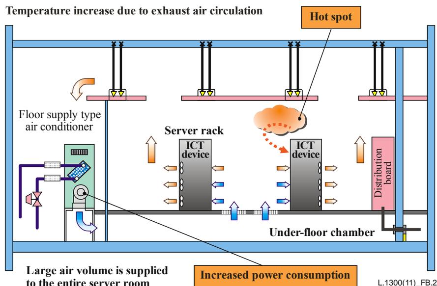
Figure B.2 – Problems with typical air conditioning
