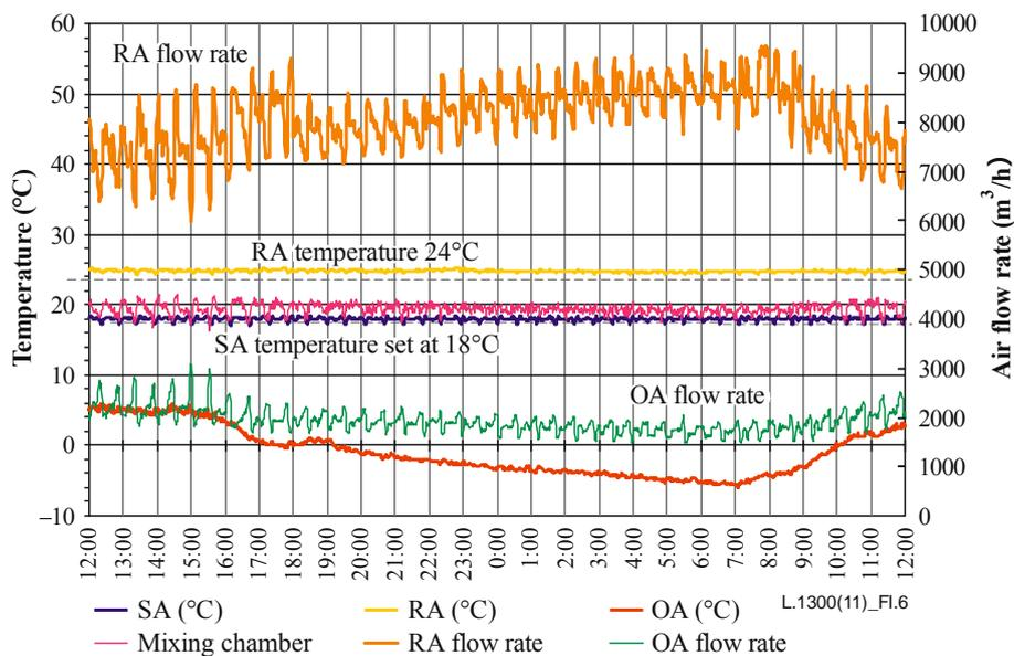
**Figure I.6 – Air temperature and airflow rate**
