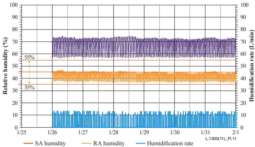
**Figure I.11 – Relative humidity of air and the humidification rate**
