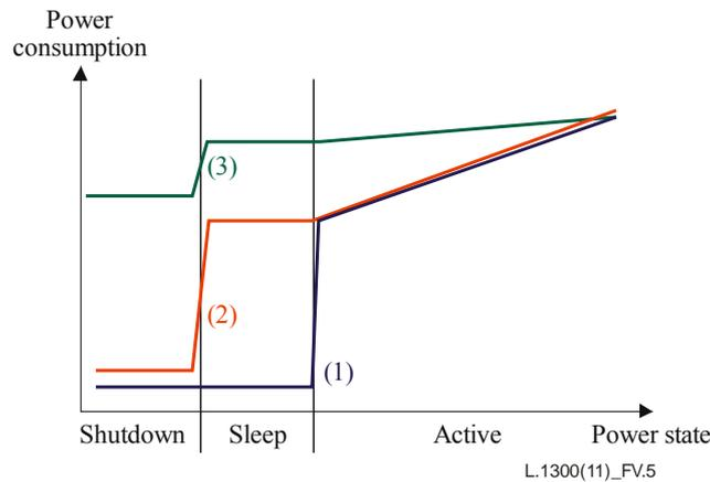
**Figure V.5 – Power patterns due to the power state of ICT equipment**
