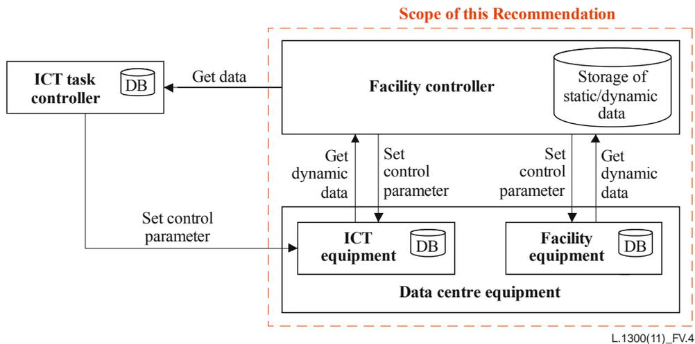
**Figure V.4 – Example of control architecture**
