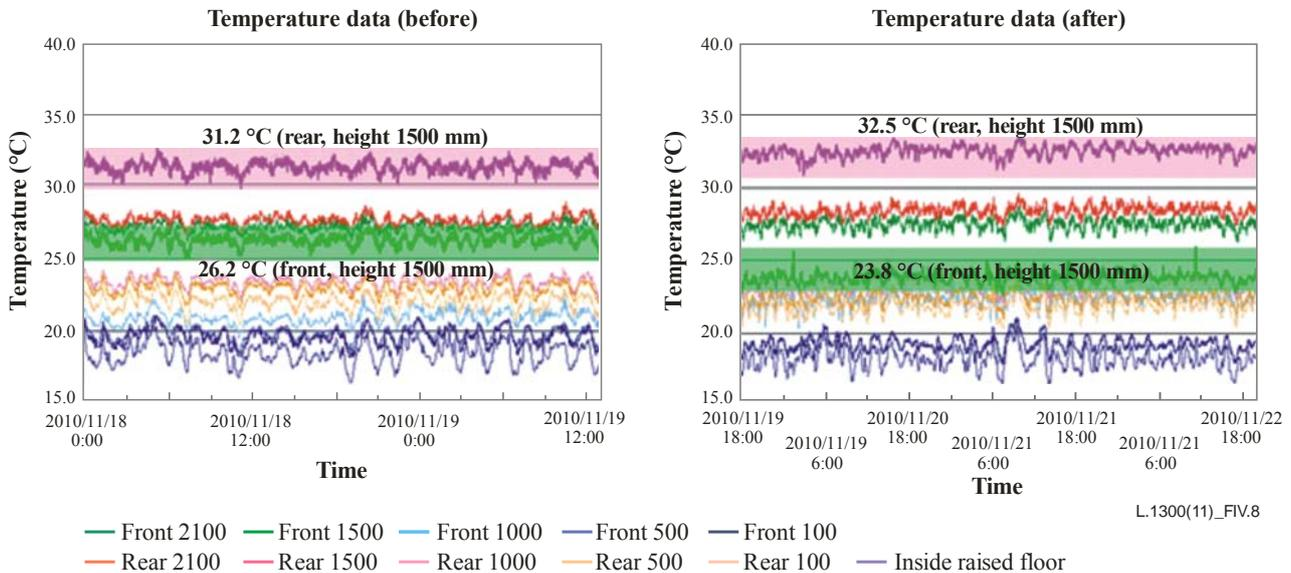
**Figure IV.8 – Results of Rack 1 after installing a duct at the outlet**
