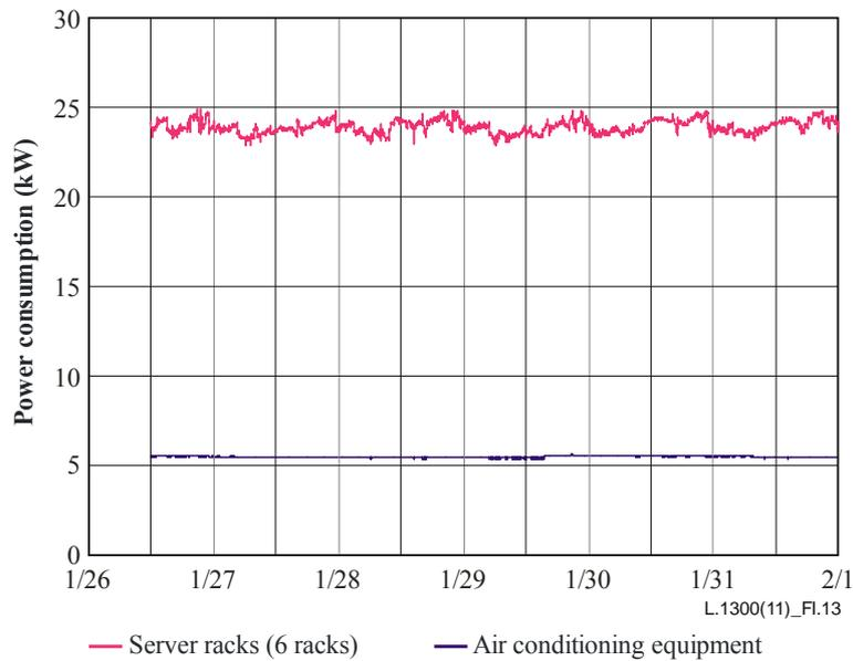
**Figure I.13 – Power consumption of servers and air conditioning equipment (snow and ice cooling)**
