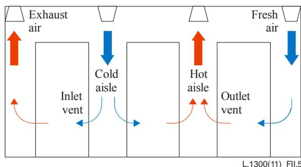
**Figure II.5 – Schema of air distribution according to configuration 1**
