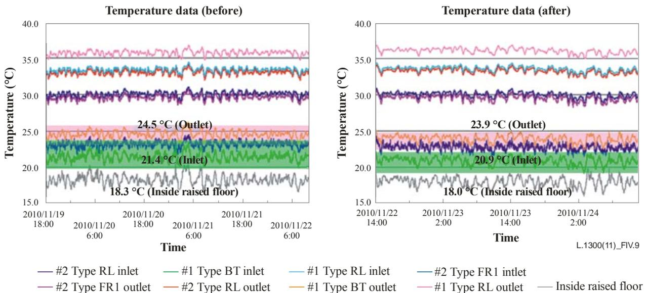
**Figure IV.9 – Results of Rack 1 after installing a duct at the outlet and at the inlet**
