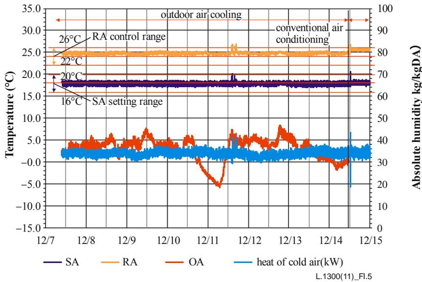
**Figure I.5 – Air (SA, RA, OA) temperature and heat energy**
