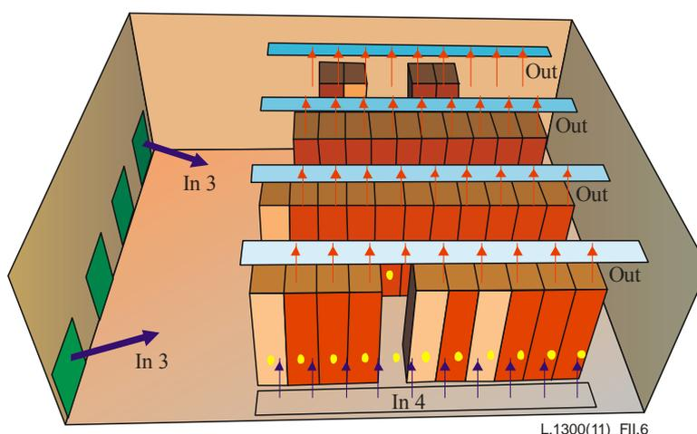
**Figure II.6 – Schema of air distribution in scenarios 3 and 4**
